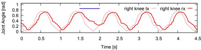
Fig. 3: Commanded (tx) and measured (rx) joint angles of the right knee during walking in place. To demonstrate the joint elasticity, the robot was pushed down on the right hip at 1.5 seconds. The blue bar indicates the time of the push. The position tracking error increases significantly in this phase.
