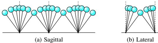
Fig. 4: Stick diagrams of a compass gait. (a) In the sagittal direction, the center of mass crosses the pendulum pivot point in every gait cycle. (b) In the lateral direction, the center of mass oscillates between the pivot points.
