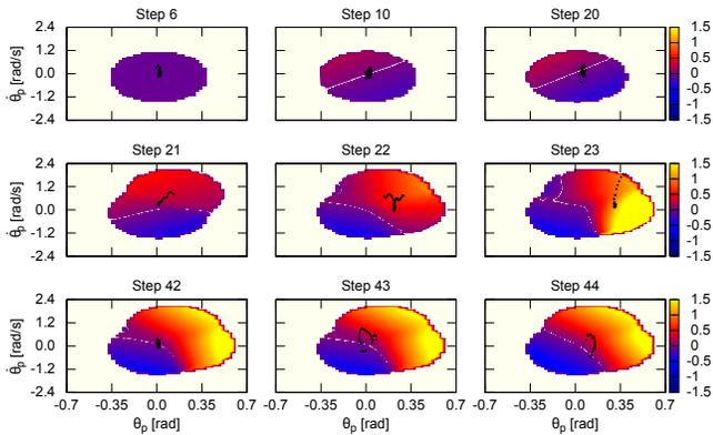
Fig. 8: Evolution of the learned feedback controller during the push-recovery experiment. The black dots mark the data points that were used to update the function approximator at the end of the step.
