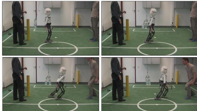
Fig. 1: Humanoid robot Copedo regains its balance after a strong push from the back.
