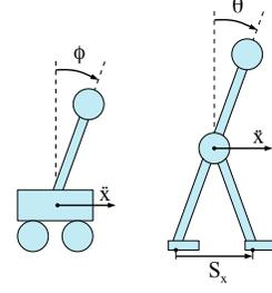
Fig. 5: The pendulum-cart model (left) resembles the angular dynamics of a biped (right). When the cart accelerates, the pendulum angle is accelerated in the negative direction. A biped accelerates by increasing its step size and can counteract undesired angular momentum.
