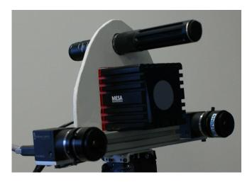
Fig. 2. Sensor setup used in our experiments. A MESA SR4000 camera and PointGrey Flea2 13S2C-C cameras acquire depth and color images. The sensor head is mounted on a pan-tilt unit.
