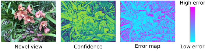
Fig. 6. The confidence predicted by the network is low near depth discontinuities where occlusion occur and therefore errors are likely.
