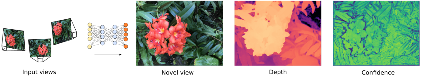
Fig. 1. NeuralMVS processes multiple input views to synthesize a novel colored view with corresponding depth and gives an estimate for the output confidence.
