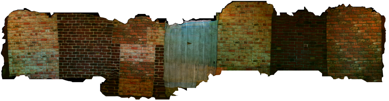
Fig. 10. 2D visualization of the chimney walls. Reconstructed surface of seven walls from the mock-up chimney shown in Fig. 1. Despite some warping effects caused by the unwrapping of the 3D structure, all details are accurately reconstructed.
