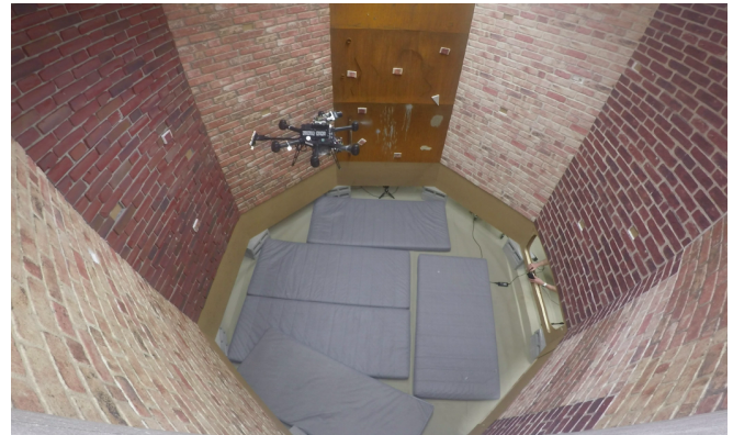
Fig. 1. Autonomous chimney inspection. Our lightweight chimney inspection MAV navigates autonomously assisted by real-time 6D laser localization and fast visual odometry. A double spiraling scan pattern facilitates good coverage and loop closing for camera-based surface reconstruction of the chimney walls. Our MAV is evaluated in a chimney mock-up resembling wall structures found in real industrial chimneys.
