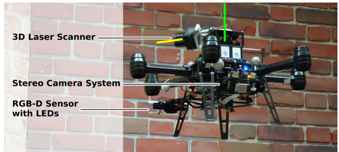
Fig. 2. Sensor setup. Our MAV is a hexarotor equipped with a rotating 3D laser scanner for localization and obstacle avoidance, a stereo camera system for visual odometry estimation, and a high-resolution camera for surface reconstruction. For better illumination and shorter exposure times, the scanned wall is illuminated by bright LEDs. The 2D laser beam rotates around the yellow axis yielding laser scan lines. The laser scanner rotates around the green axis to accumulate scan lines to full 3D scans.
