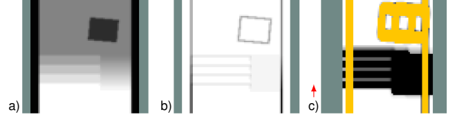
Fig. 9. Level 2 : a) height map, b) height difference map, c) foot area pair cost map for the orientation indicated by the red arrow.
