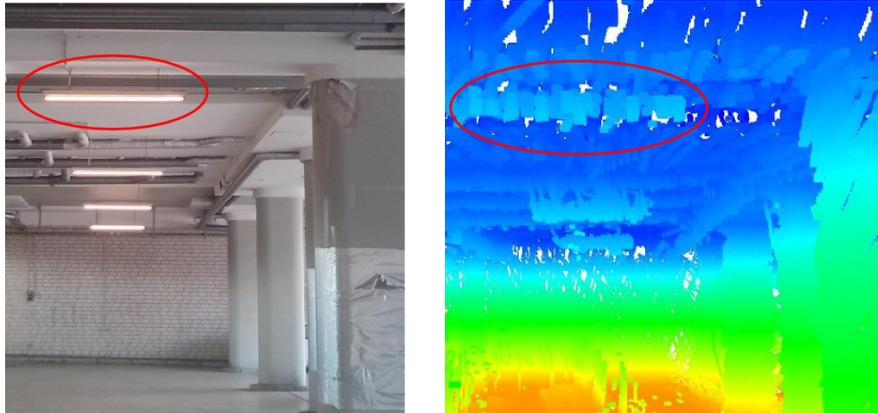
Fig. 8: The structure of the ceiling showing hanging lamps in a photo (left) and the resulting 3D map (right).
