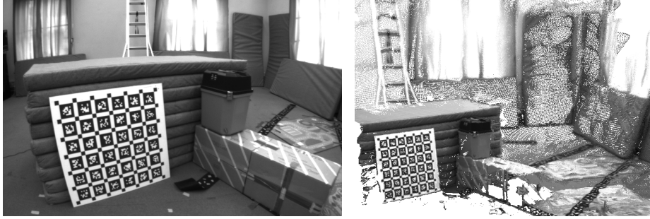
Fig. 6: Left: Camera image. Right: Reconstructed semi-dense 3D point cloud.
