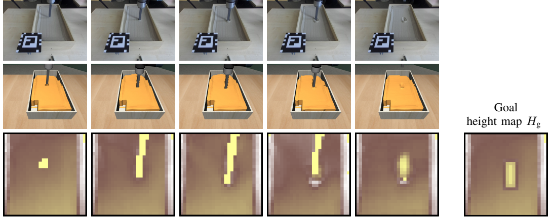
b) We deploy the agent to the real robot in a zero-shot manner, without any additional training. From top to bottom, we show the raw camera view of the box filled with the granular medium, the reconstructed 3D scene in simulation, and the reconstructed height map that the agent observes, while it manipulates the granular medium to match the desired goal configuration. Note that the granular medium is not perfectly flat like in the simulated scenario. Despite noisy observations from the depth camera, the agent is able to create the desired rectangle shape in the real world.
