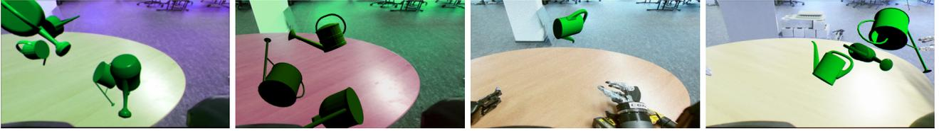
Fig. 5. Synthetic training scenes for semantic segmentation and 6D pose estimation.
