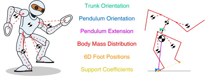
Fig. 1. Approximation of a humanoid body and its limbs with triangles. The approximation allows to parameterise a whole body pose with only a few parameters to produce balanced motions.
