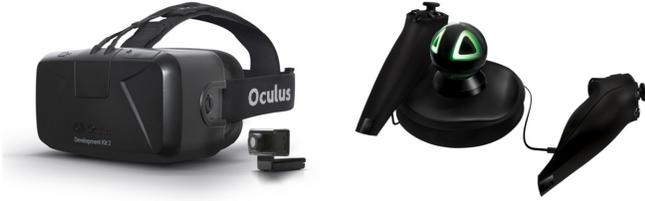
Fig. 3: Upper-body operator interfaces: Left: Oculus Rift DK2 HMD. Right: Razer Hydra 6DoF controllers.
