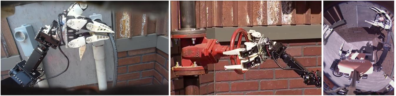
Fig. 5: Left: Inserting the plug as seen from the right hand camera. Middle: Momaro turns the valve. Right: Flipping the switch as seen from the top-down camera.
