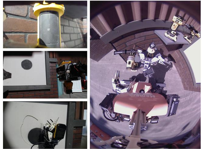
Fig. 6: Top Left: Grasping the cutting tool as seen from the right hand camera. Right: Same scene as seen from the top-down camera. Middle Left: Grasp used to switch on the tool. Bottom Left: Momaro cutting the drywall as seen from a sensor head camera.
