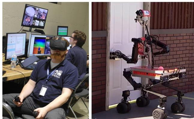
Fig. 1: Intuitive teleoperation. Left: Upper (front) and lower body (back) operator. Right: Momaro opening the door.
