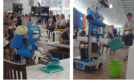
Fig. 7. Sweeping dust using a pan and a brush. Our robot Cosero estimates the pose of the dust pan and the brush to grasp them (left). It pours the content of the dust pan into a dust bin (right).
