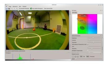
Fig. 7. Color calibration tool used to generate YUV color lookup tables.
