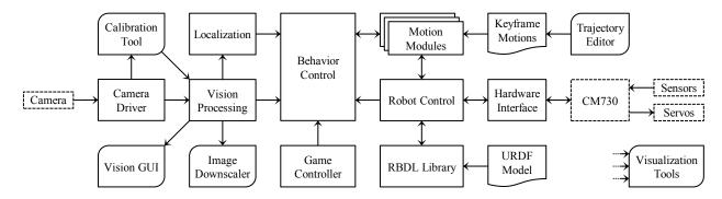
Fig. 3. Diagram of the NimbRo-OP ROS framework software architecture. Boxes with a dashed outline represent hardware elements, boxes with rounded corners represent auxiliary software tools that are not necessarily required for execution of the framework, and the arrows show the flow of information. Boxes with a wavy lower edge represent data files. The visualization tools use information from throughout the entire architecture.
