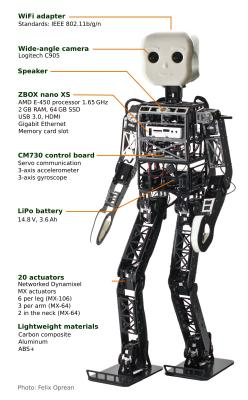
Fig. 2. Diagram of the NimbRo-OP robot hardware.
