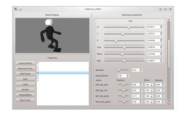
Fig. 5. Screenshot of the trajectory editor, used to generate and edit the keyframe motions used by the motion player.
