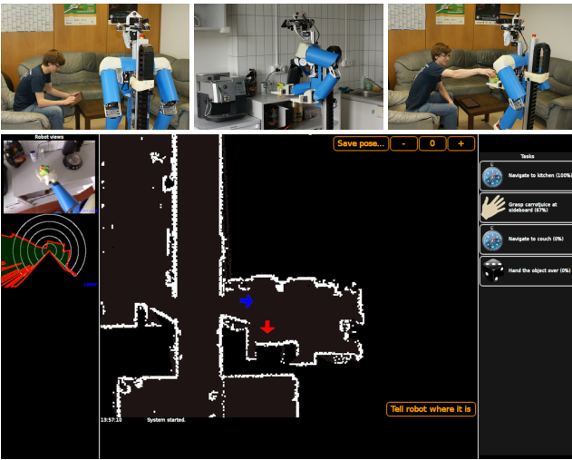
Figure 2: Illustration of our task-level teleoperation interface. Top left: A user composes a task. Bottom/top middle: The robot grasps an object. Top right: The robot delivers the object.
