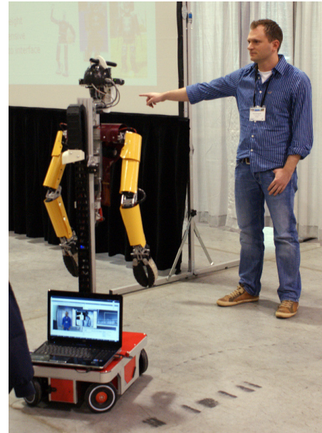
Figure 1: Application scenario from ICRA 2010 Mobile Manipulation Challenge. Our robot approaches the user and he selects a drink by pointing to it.
