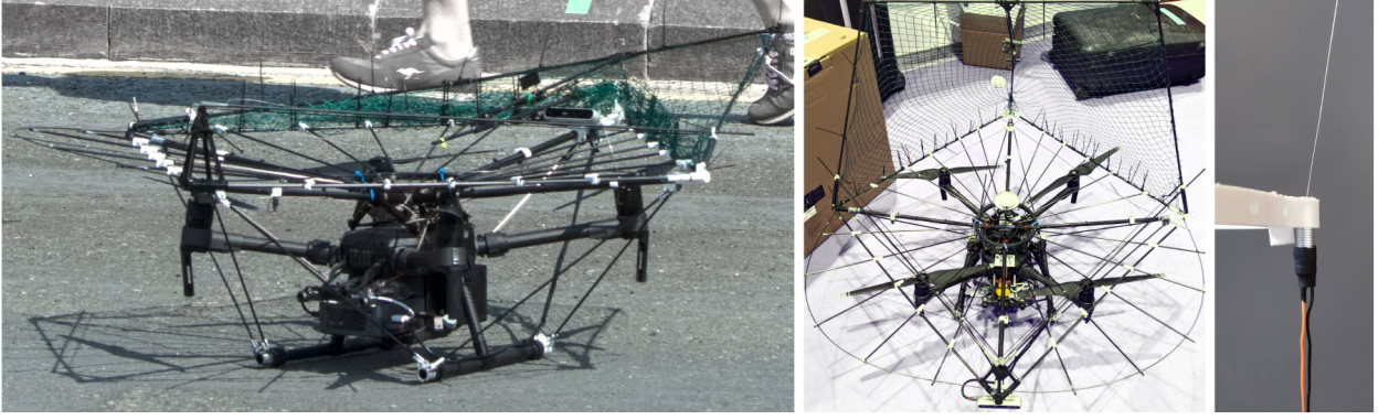
Figure 16: Design of our UAV “Chaser” equipped with a foldable net to capture the target, a fast onboard computer, an Intel® RealSense™ D415 camera and a Google Edge TPU.
