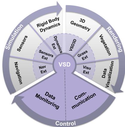
Fig. 6. The micro-kernel design pattern of the eRobotics system. Plugins can extend functionalities with new algorithms and self-defined database elements.
