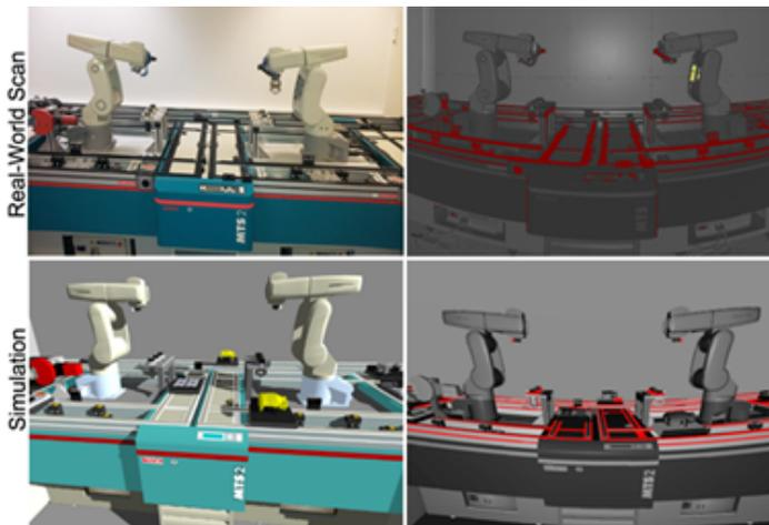
Fig. 10. Comparison of a real world and a simulated intensity image of a 3D LiDAR scan of a robot workcell. Areas marked in red illustrate scanning errors.
