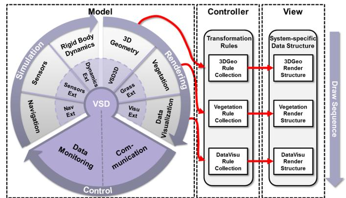
Fig. 8. Illustration of the system's micro-kernel architecture in combination with the MVC design pattern. Plugins can extend functionalities with new algorithms and self-defined database elements. Defined rules transform the semantic graph into system-specific data structures for efficient rendering.
