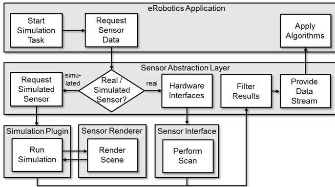
Fig. 9. A hardware abstraction layer is used to decouple application development from the applied sensors, regardless if real world or simulated ones.
