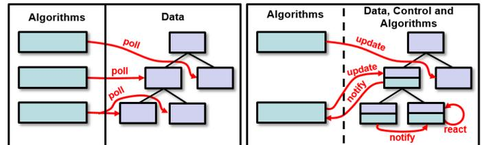
Fig. 5. Left: common, passive system structure. Plugins provide algorithms that poll data stored in the database. Right: system based on an active, event-driven database.
