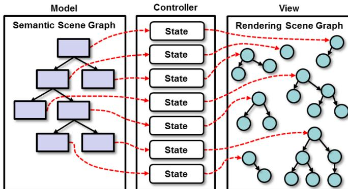
Fig. 7. Illustration of the split scene graph approach to separate semantic from rendering data, following the Model-View-Controller (MVC) design pattern.
