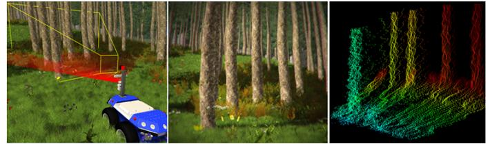
Fig. 11. Simulation of the Seekur Jr mobile robot platform equipped with a 2D LiDAR scanner, a stereo camera and a ToF camera for virtual testing and development of navigation and mapping approaches.
