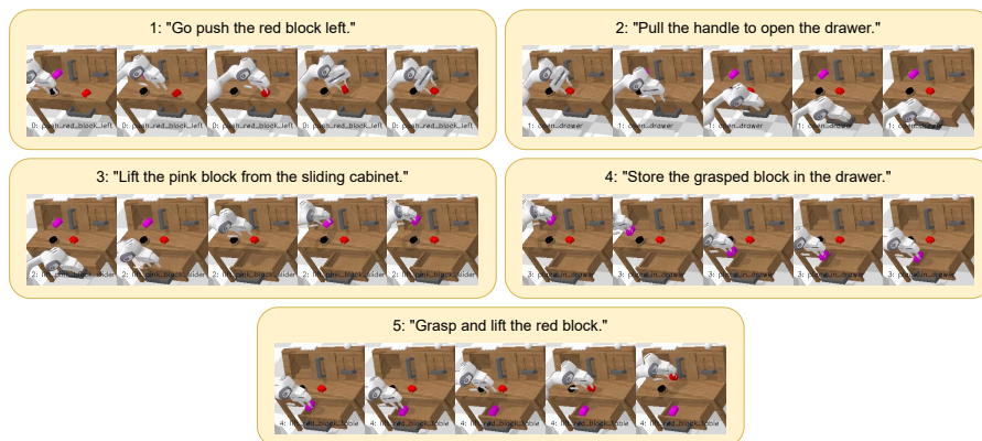
Fig. 2. EL3DD executing a task chain during evaluation. All 5 tasks were successfully executed in a row.
