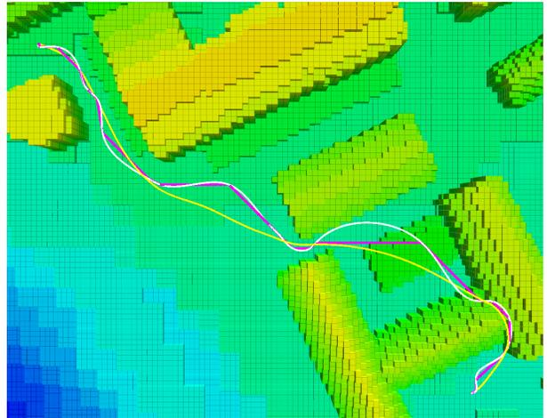
Fig. 1: Exact planning of smooth trajectories with velocity and acceleration dimensions for MAVs is often not feasible fast enough needed for frequent replanning. We plan coarse 3D trajectories (pink), incorporate simple assumptions about the MAV’s dynamics (white), and optimize this initial guess quickly to obtain a least cost kinodynamic trajectory (yellow) w.r.t. distance to obstacles and control costs.
