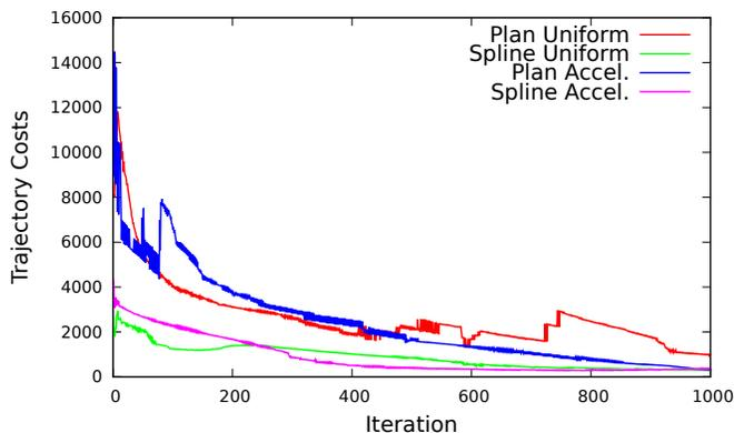
Fig. 7: Trajectory costs (state and control costs) per iteration of the optimizer. Whereas the optimizer converges to nearly the same value for all initializations, spline-based initializations (green/pink) reach a low value much faster. Also the combination of spline-based initialization with non-uniform accelerations (pink) reduces the convergence time.
