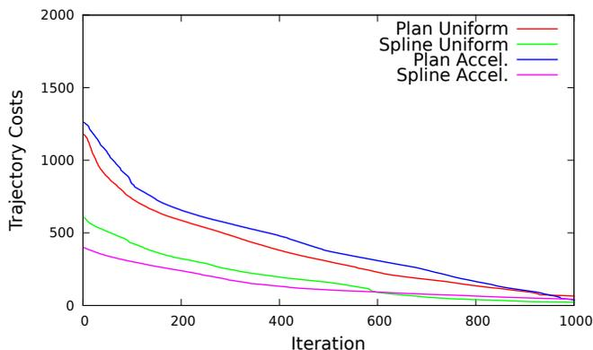
Fig. 8: Summed control costs per iteration of the optimizer. After initialization the overall control costs of the trajectory could be reduced by 25 - 34% by employing better timings and by approx. 75% by using splines in this example.
