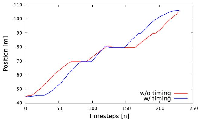
Fig. 3: Uniform plan discretization (red) vs. discretization according to motion model (blue) of the MAV’s trajectory in the  $x$ -coordinate. Discretizing according to a motion model facilitates faster convergence of the trajectory optimizer.
