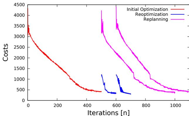
Fig. 10: Frequent reoptimization allows for quick reactions on deviations while following a trajectory. The initial trajectory is planned and optimized for 500 iterations (red). Reoptimizing the old trajectory yields a close-to-optimal new trajectory with fewer iterations than complete replanning.
