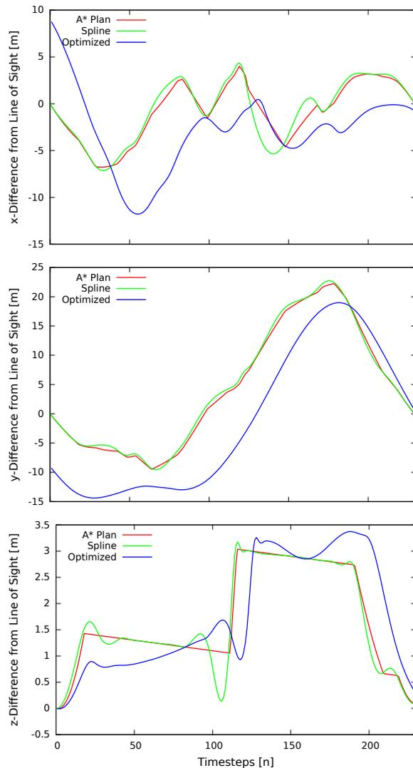
Fig. 4: Comparison of trajectories for individual position dimensions at different stages of optimization. Planned paths (red) with applied timing correction require still large accelerations when the movement direction changes. Spline interpolation (green) mitigates these effects, but tend to overshooting and are bound to the initial plans sampling points. The optimized trajectories (blue) are much smoother and reduce the necessary control effort.
