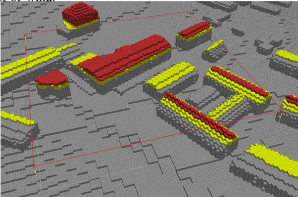
Fig. 6: OctoMap of the evaluation area. We have restricted the maximum allowed altitude for our experiments to approx. 10m over ground, otherwise flying at higher altitudes always yields shortest paths. Yellow: Obstacles influencing the MAV at 10m altitude. Red: Obstacles the MAV cannot overfly.
