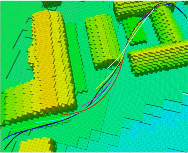
Fig. 5: We employ frequent optimization to recover from disturbances during trajectory execution. In this example the MAV follows an initial trajectory from start to goal (black). Gusts of wind push it away from the trajectory, the colored trajectories depict the newly optimized trajectories after every gust of wind.
