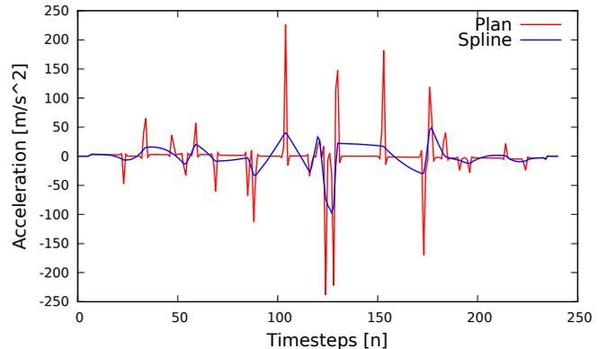
Fig. 2: Accelerations of the trajectory before optimization. Initialization with the path from a grid-based planner yields high accelerations at the connection points between plan intervals. Spline-interpolation of the path reduces these spikes yielding faster convergence.
