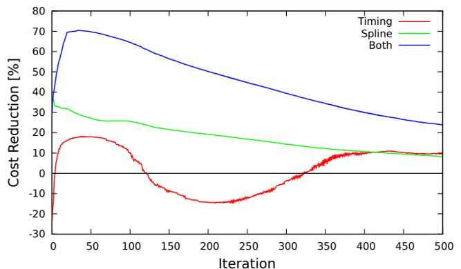
Fig. 9: Reduction of trajectory costs compared to baseline (initialization with A\* planned path) in each optimizer iteration. The results are an average over 1,216 trajectories.
