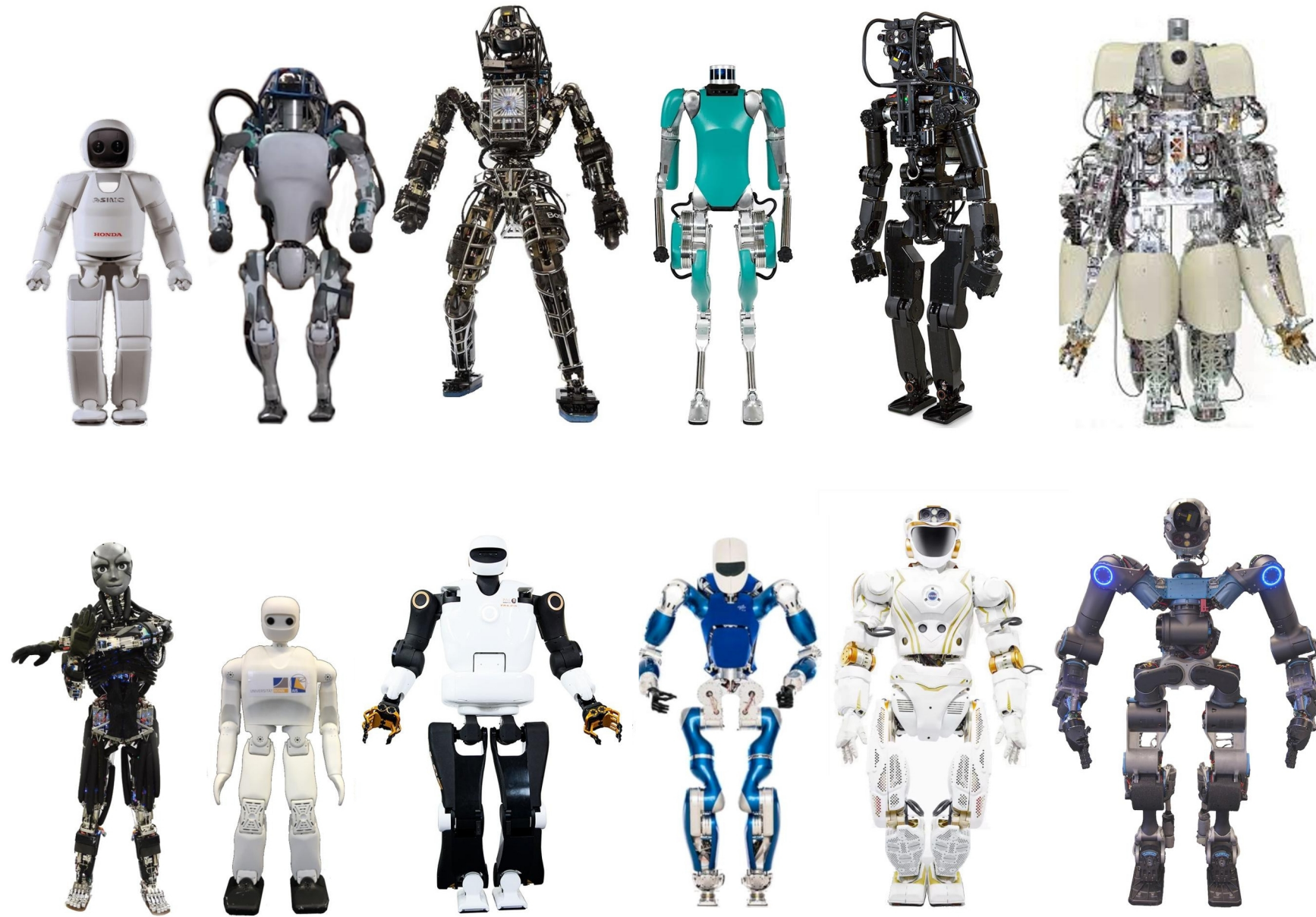
Fig. 1: Most recently developed bipedal humanoid robots with a full humanoid body plan, from left to right, top to bottom: Asimo, Atlas, Atlas-Unplugged, Digit, HRP-5P, Hydra, Kengoro, NimRo-OP2X, TALOS, Toro, Valkyrie, WALK-MAN.
