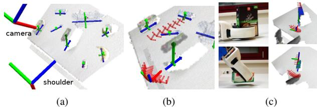
Fig. 5. Grasp planning. (a) Object shape properties. The arrows mark the principal axes of the object. (b) We rank feasible, collision-free grasps (red, size prop. to score) and select the most appropriate one (large, RGB-coded). (c) Example grasps on box-shaped objects.
