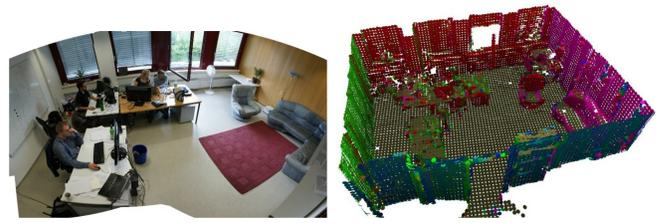
Fig. 3. Left: panorama image of an office. Right: 3D surfel map learned with our approach (surfel orientation coded by color).
