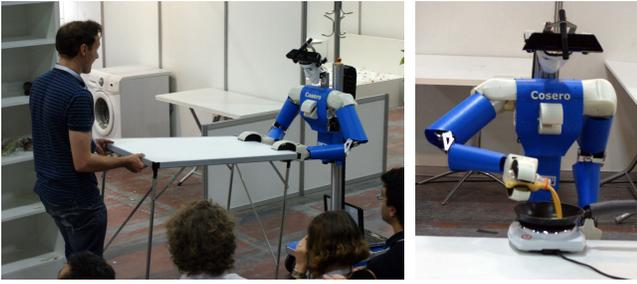
Fig. 9. Cosero cooperatively carries a table with a user and bakes omelet during the RoboCup@Home Final 2011 in Istanbul.
