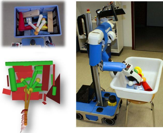
Fig. 6. Left: Objects composed from shape primitives recognized in a transport box. Right: Cosero executes a planned collision-free grasp on an object in a box.
