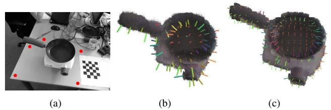
Fig. 7. Learning object models. (a) During training the user selects points (red dots) to form a convex hull around the object. (b) Color and shape distribution modeled at 2.5 cm resolution. Lines indicate surface normals (color-coded by orientation). (c) Color and shape distribution modeled at 5 cm resolution. Lines indicate surface normals (color-coded by orientation).
