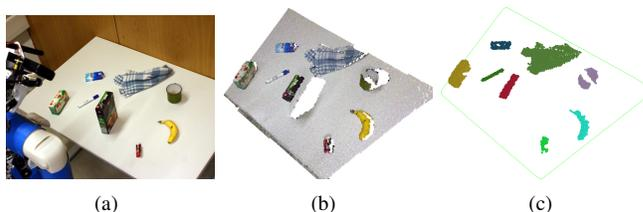
Fig. 4. Table-top segmentation. (a) Example setting. (b) Raw point cloud from Kinect with RGB information. (c) Each detected object is marked with a distinct color.
