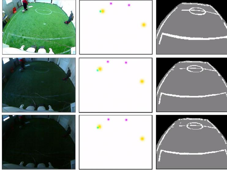
**Fig. 4.** Object detection under various lighting conditions. Left column: captured images by our robots. Middle column: output of the network indicating balls (cyan), goal posts (magenta), and robots (yellow). Right column: output of the segmentation branch showing lines (white), field (gray), and background (black).
