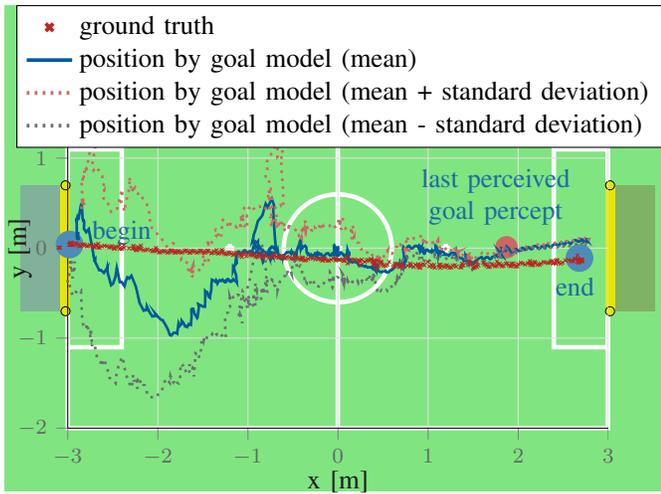
Fig. 5. The robot starts between own goal posts and walks to a ball placed in the opposing goal. The red line shows the ground truth of the robot position. Start and end points are marked accordingly. The blue graph shows the position of the robot calculated by a simple triangulation based on the MHGM and averaged over 10 runs. The dotted lines illustrate the corresponding standard derivation of the robot position. The point of the last perception of a goal post is also marked.
