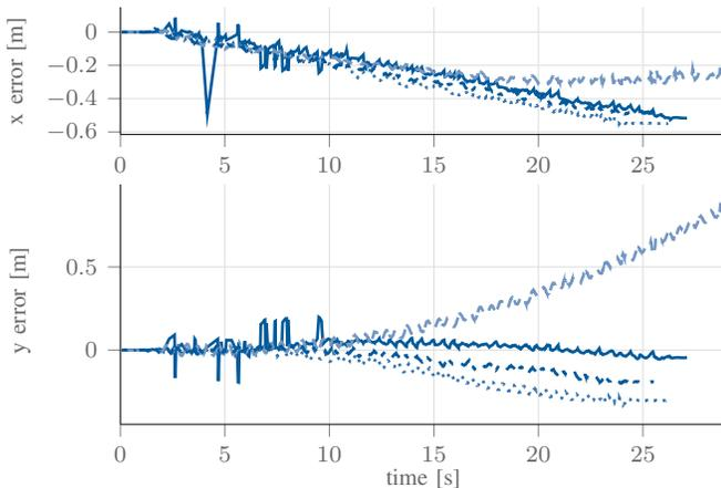
Fig. 2. In this experiment, four robots are forced to walk a straight line. The  $x$  and  $y$  components of the path traveled by each robot (odometry) are plotted separately over time.
