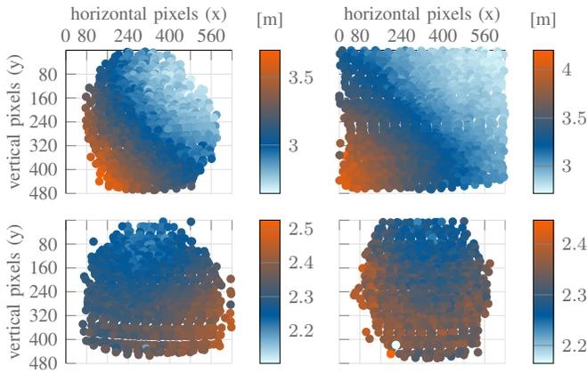
Fig. 1. Estimated distance to a goal post depending on its position in the image. The actual distance is 3m. The robot moves only its head to ensure the goal post is detected accurately, the head speed is very slow. Each point represents a goal post detection in corresponding image coordinates with the color illustrating the estimated distance to it. The results for four different robots are shown.
