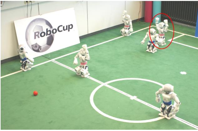
Fig. 5. Field configuration used in the timing tests with camera support. The planning is performed on the red circled robot. The orange ball marks the target.
