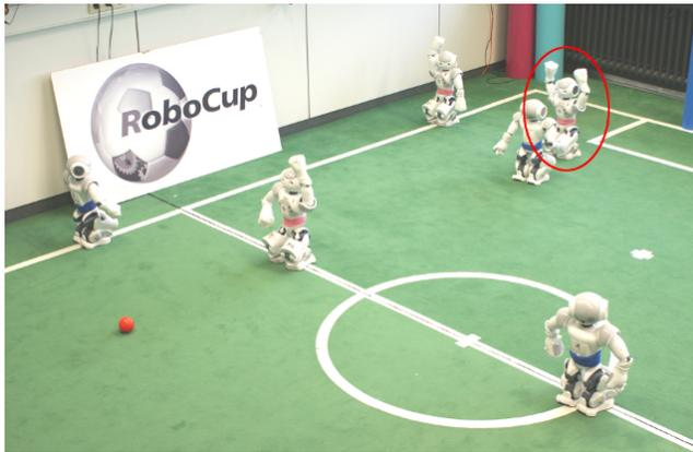
Fig. 5. Field configuration used in the timing tests with camera support. The planning is performed on the red circled robot. The orange ball marks the target.
