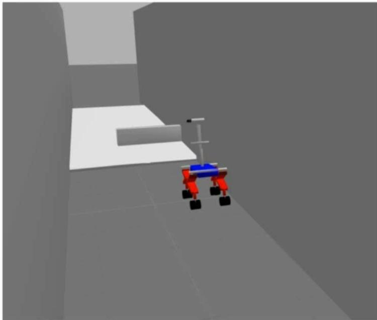
**Scenario:** Momaro has to step up a height difference and manoeuvre around a small wall.
