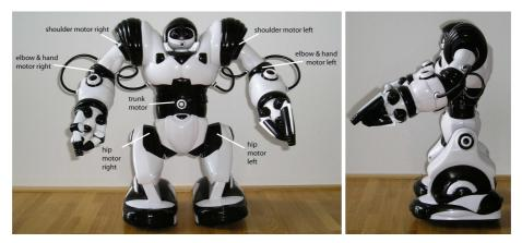
Fig. 1. Robo Sapien. Left: frontal view, seven motors move the robot. Right: side view.
