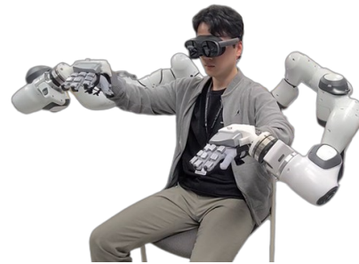
Fig. 3: A proposed bimanual haptic display combined with a haptic glove and a VR headset
