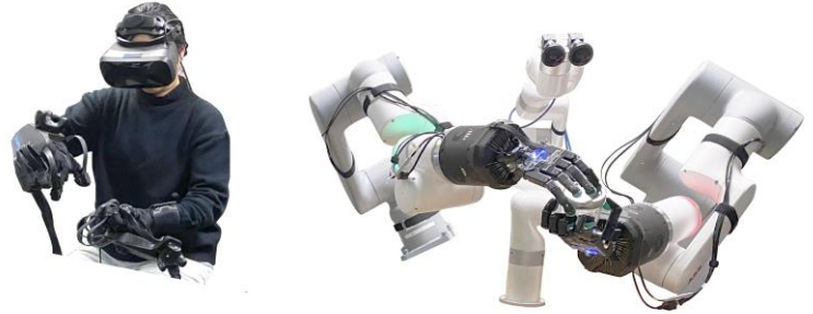
Figure 1. Dexterity Testbed Nexus. Left: Operator station, right: Avatar station. Only the upper limbs are tracked and mirrored. Feedback is provided to the user visually and haptically.
