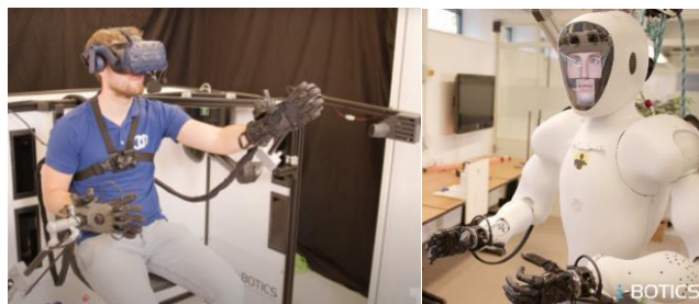
Figure 1: On the left: the operator control pod. On the right, the robotic avatar.
