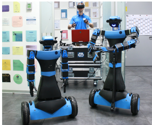
Fig. 1: Alter-Ego Platform: Alter-Ego (on the left), Alter-Ego X (on the right) and the pilot station (in the middle).
