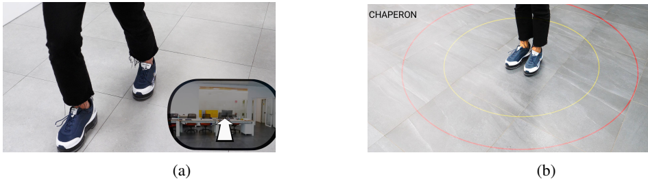
Fig. 3: In (a) an example of intention-detection together with the headset visual feedback. In (b) the "chaperon", in yellow the first safety zone is depicted meanwhile the red circle shows the zone outside which the robot movements are stopped.
