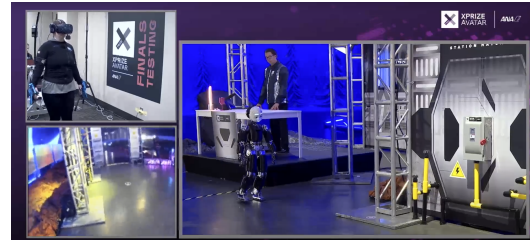
Fig. 4: The robot walking and the judge wearing the sensors and controlling the robot via the iFeel Walking.
