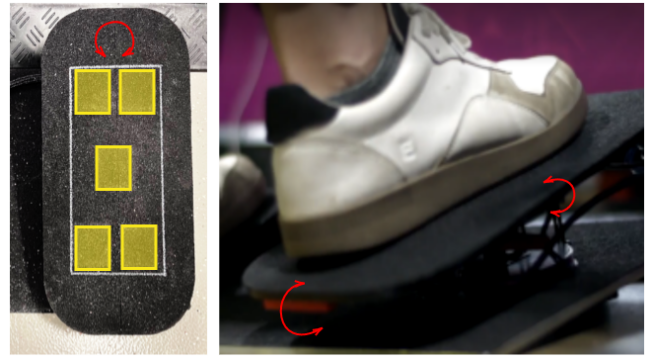
Fig. 4: Top view and side view of the 3D footplate. The red arrows denote the possible control direction. The yellow boxes denote the locations of the underneath pressure sensors.
