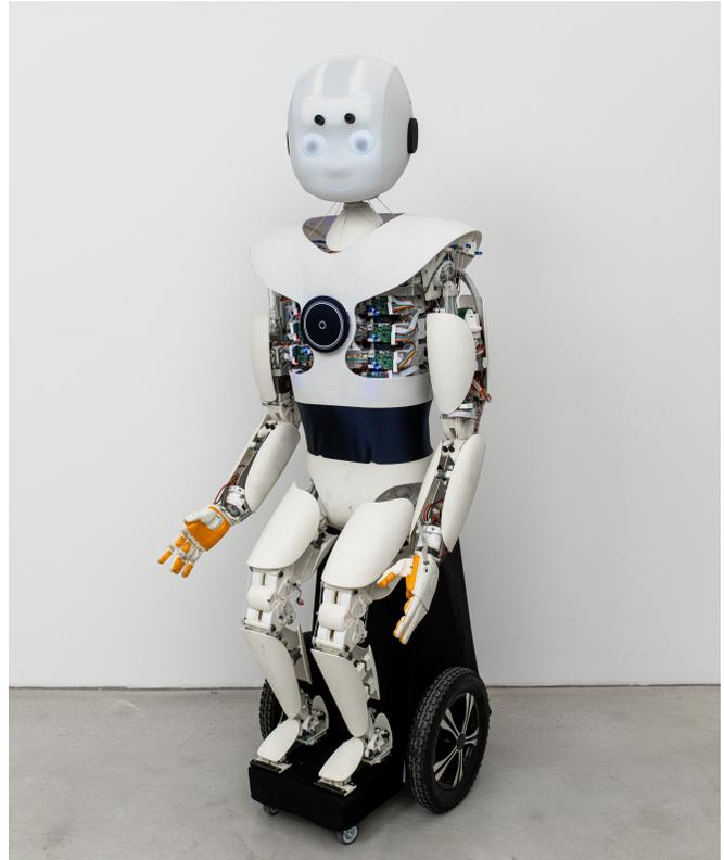
Fig. 1. Tendon-driven humanoid robotic avatar Robody
