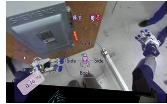
Fig. 5. Interface for walking, motion and field of view retargeting.
