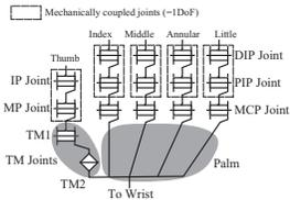
Fig. 2. Kinematic diagram of D-Hand v3
