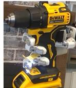
Fig. 4. D-Hand v3 operating drill
