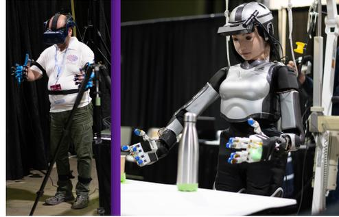
Fig. 1. HRP-4CR synchronized with the operator
