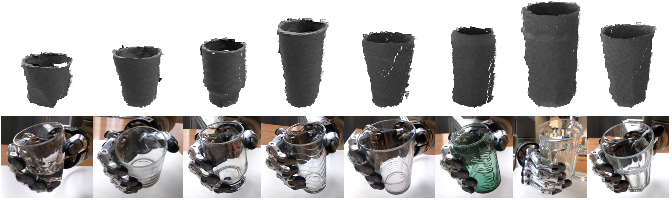
Fig. 9. Training instances for the synergy learner. Top: observed point clouds of the objects to be grasped, and bottom: the respective grasped performed through teleoperation.
