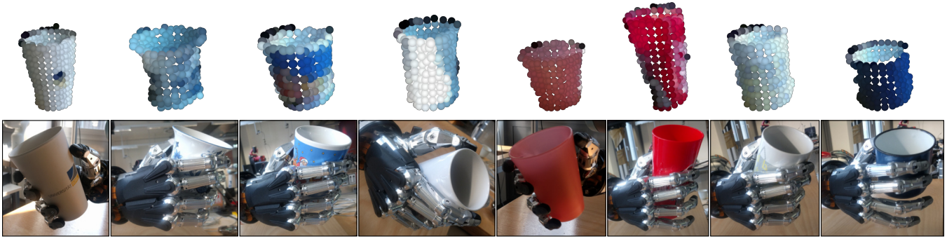
Fig. 12. Real robot experiments for the Glass category. All the objects were presented for the first time to the system and they were successfully grasped.
