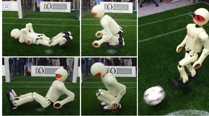
Fig. 3. Dynamic get-up motions, from the prone (top row) and supine (bottom row) lying positions, and a still image of the dynamic kick motion.
