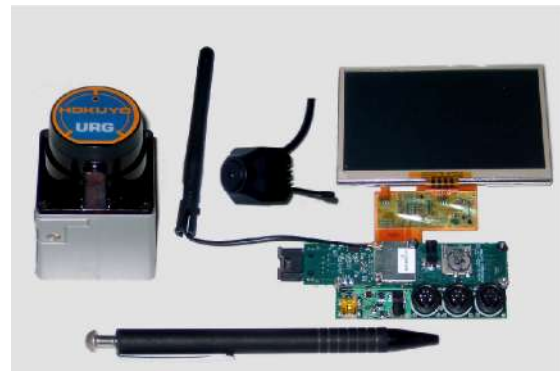
Figure 13. From the left to the right a HOKUYO URG-04lx laser range-finder, a wireless visortech GP-811t camera and Gumstix Verdex XL6P computer with 802.11 (g) wireless communication module are shown. The display is detachable and is not needed during the flight.
