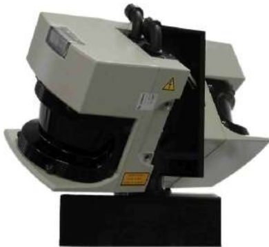
Figure 5. The continuously rotating laser scanner 3DLS-K2 consists of a rotation unit with 2 SICK-LMS laser scanners.
