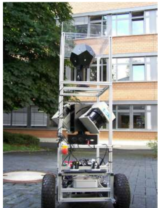
Figure 1. First evaluation of the UGAV. The ground platform is built of a Volksbot RT3 which is equipped with batteries, vision sensors, 3D laser scanner, control computers and a landing platform on top for the quadrotor
