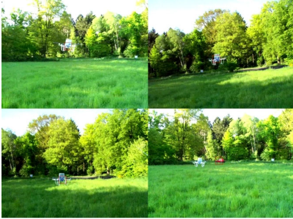
Figure 11. Most salient regions in four frames of the quadcopter flight. In more than 80% of the images is the quadcopter the most attentive object. When a red car drives through the scene the attention goes to it (bottom right).
