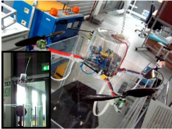
Figure 14. A prototype of the quadrotor used for the evaluation. On the bottom-left figure the copter is tested for landing on a small platform in the Fraunhofer IAIS robotic laboratory.
