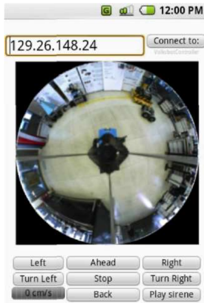
Figure 9. User interface of teleoperator software in the android environment.
