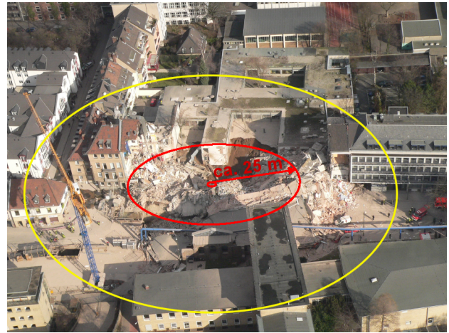
Fig. 3. Aerial view of the scenery on arrival of the first rescue units. The red circled area shows the "hot zone" with a pit diameter of about 25m [1]. The yellow circled area shows the restricted access area only for rescue personnel.
