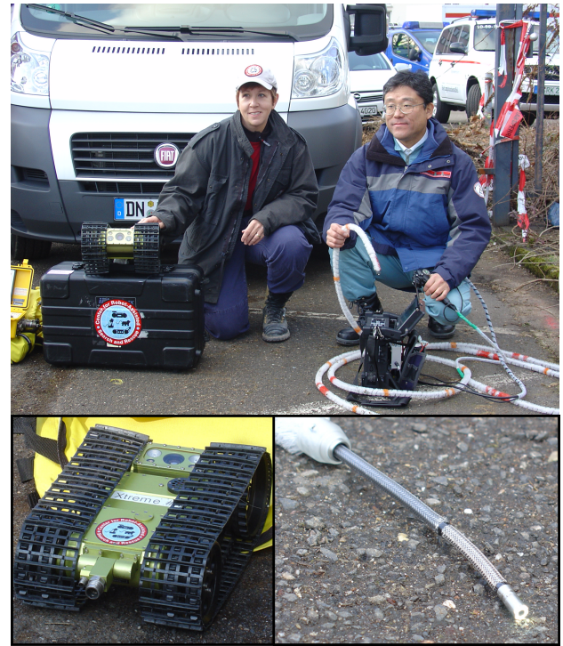
Fig. 7. On the left side Dr. Robin R. Murphy with the VGTV Xtreme and on the right side Dr. Satoshi Tadokoro with the Active Scope Camera (ASC) .
