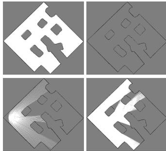
Figure 3: Using frontier-based exploration for inspection. From left to right: fully explored environment, cleared free space, and the map after the first update and after 50% inspection time.
