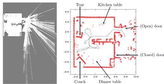
Figure 6: Exploring a real-world environment (the RoboCup@Home arena at the GermanOpen 2009). Left: final map, right: trajectory of the robot.
