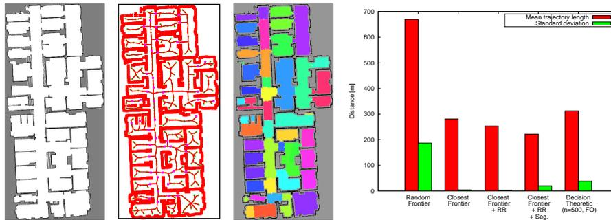
Figure 2: Map segmentation for roomwise exploration. Shown are (from left to right): the (final) input map, the Voronoi diagram with the critical points, the refined segmentation, and the measured path lengths for the different strategies (*RR*. = repetitive re-checking, *Seg.* = map segmentation).
