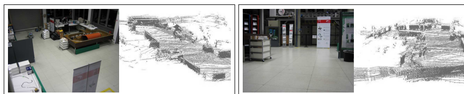
Figure 2: Two views on a generated 3D model being constructed by matching the generated point clouds. The height of the built model corresponds to the height of the robot and thus to that of the area of interest.
