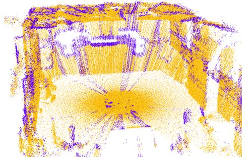
**Fig. 6:** Accumulated 3D scans of an indoor environment. Measurements from first echo (yellow) and the second echo (purple). In case of partial occlusions, e.g., by the MAV itself, multi-echo detection leads to an increase of distance measurements.
