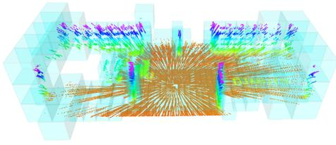
**Fig. 9:** A grid-based local multiresolution map with a higher resolution in the close proximity to the sensor and a lower resolution with increasing distance. The point colour encodes the distance from the ground.
