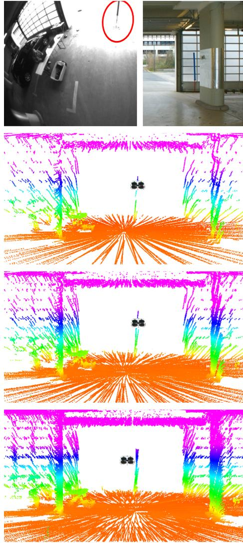
**Fig. 13:** Aggregating 3D scans in a scene of the third experiment. Photos show the sensed pole (red ellipse) and the surroundings from an on-board camera with fish-eye lens (top left) and an external camera (top right). Scan aggregation increases the detection probability and the point density in the map (from top to bottom: map after aggregating 5, 10 and 20 scans).
