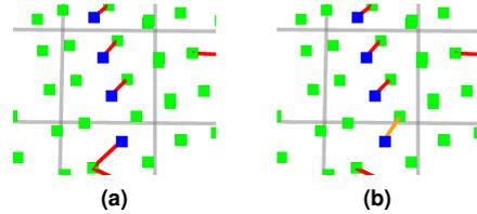
**Fig. 10:** Assigning point correspondences. (a) For every point of a 3D scan (blue), a corresponding map point (green) is initially assigned from the cell’s point list (red line). (b) If the distance to neighbouring cells is smaller than the distance to the initial assignment, closer points might be found in the neighbouring cell (orange line).
