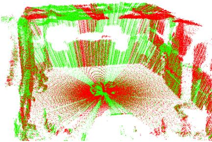
**Fig. 5:** Accumulated 3D scans of an indoor environment. The colour encodes the different half rotations of the scanner. Moving the optical centre of the 2D laser range finder away from the rotation axis of the actuator results in different self-occlusions of the scans from the first (green) and the second (red) half rotation.
