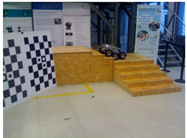
Fig. 2: The scene of the first experiment carried out in the Robotic Pavilion at Fraunhofer IAIS, Sankt Augustin. The scene consists of a wooden staircase with a robot on it, some posters and a calibration pattern. The robot moved on a square with 120 cm side length.
