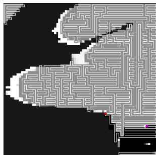
Figure: Occupancy Grid After 250 Measurements
