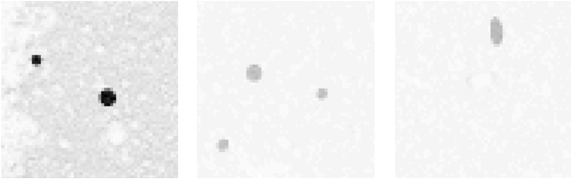
Figure 5.4: Example horizontal slices of combined crops virtual root and real soil. Darker spots in the images are cross sections of the root branches.
