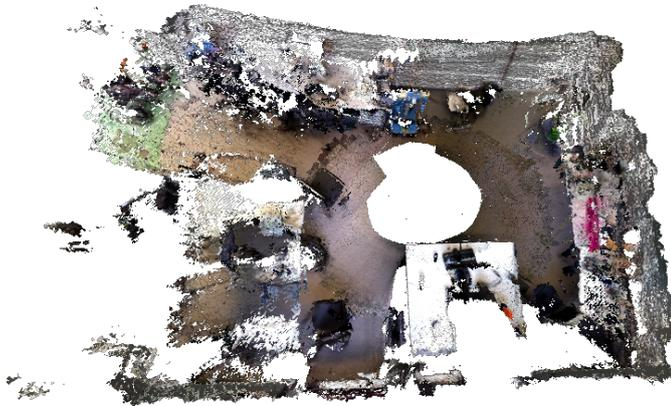
**Figure 7.7:** Resulting mesh of the CSLAM with the Robotics Lab dataset without the undefined registrations detector.
