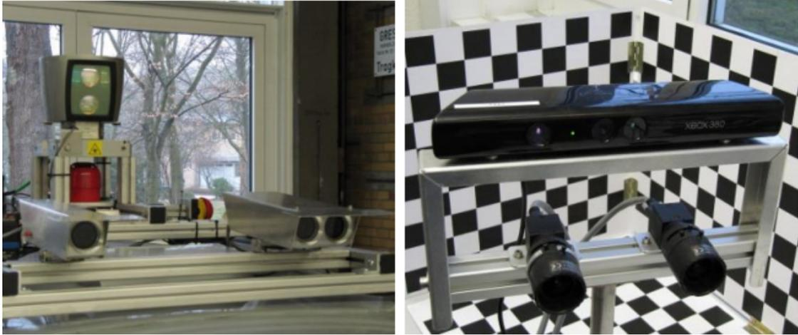
**Figure 1.2:** Experimental set-up with multiple cameras and a checkboard pattern from Geiger et al. (2012)
