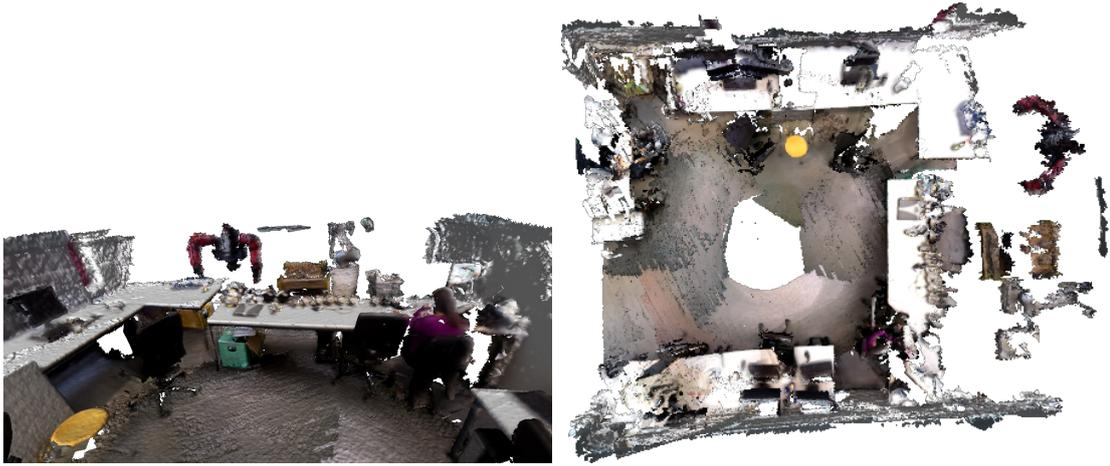
**Figure 7.5:** Resulting mesh of the CSLAM with the Graphics Lab walking dataset.
