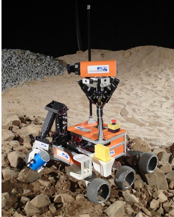
**Figure 6.1:** Explorer robot with eight RGB-D sensors used for the experiments.
