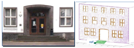
Figure 2.7: An example of a simple staircase that consists of a single flight of stairs. We can also notice the reference point at the bottom left corner of the flight of stairs as defined by Plümer which describes the origin point in the stairs model. Using this global reference point and the other attributes mentioned in this section, a stair model is defined as a part of buildings modelling (source: [39]).
