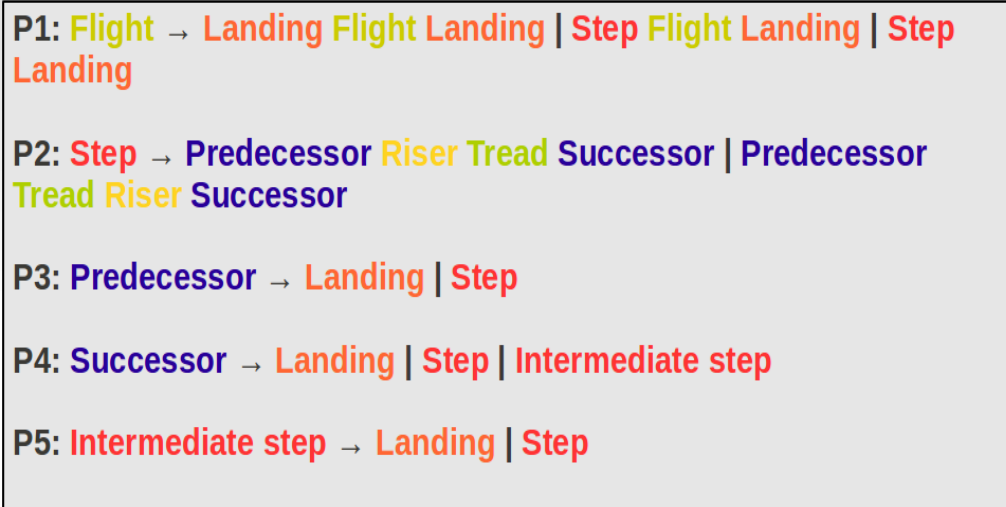
Figure 4.3: Our own defined grammar. This grammar is modified from the original definition of Plümer’s grammar in section 2.4 to include Landing (P1) and predecessor and successor (P2), definition of predecessor (P3) and successor (P4) and definition of an intermediate step (P5).
