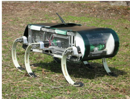
Figure 2.3: RHex robot developed by Boston Dynamics. As can be seen it is a six legged robot with a stereo camera at the front (source: [50]).
