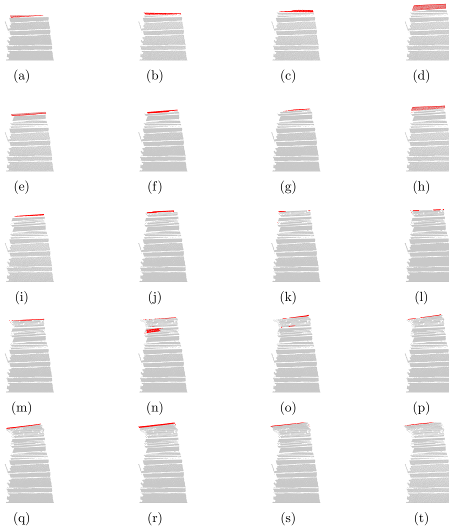
Figure 5.4: Updating the incremental model in a going upstairs perspective. The red points represent the newly added points. In reality building each of these models requires 100-120 input clouds but for the sake of visualization only images with the highest number of added points are shown.
