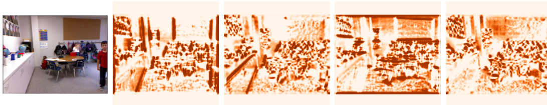
Figure 3.6: The HOG channels corresponding to four directions. The color intensity represents the magnitude of the gradient, white means zero intensity.
