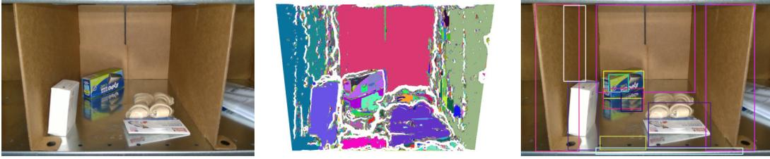
Figure 5.6: RGB-D based additional region proposals. Left: RGB frame. Center: Regions labeled using the connected components algorithm. Right: Extracted bounding box proposals.
