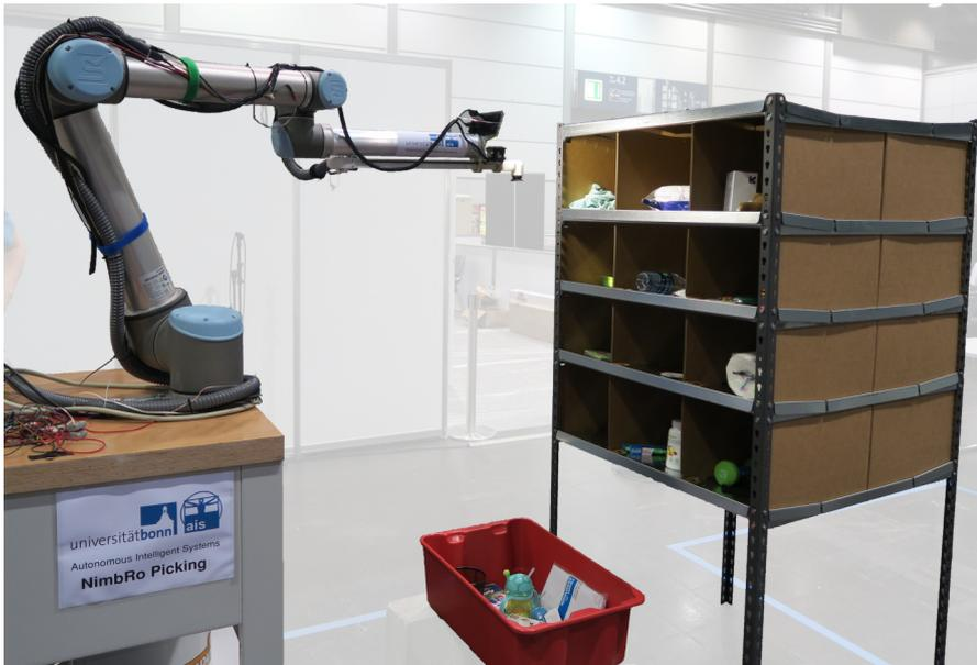
Figure 4.1: Team NimbRo's robot at the APC 2016, showing the entire work cell layout with shelf, tote, and robot.
