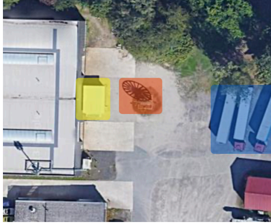
Figure 4.8: Clutter not represented in model include trees, cars (blue), a large gearwheel (red), and the hut (yellow), taken from [23]
