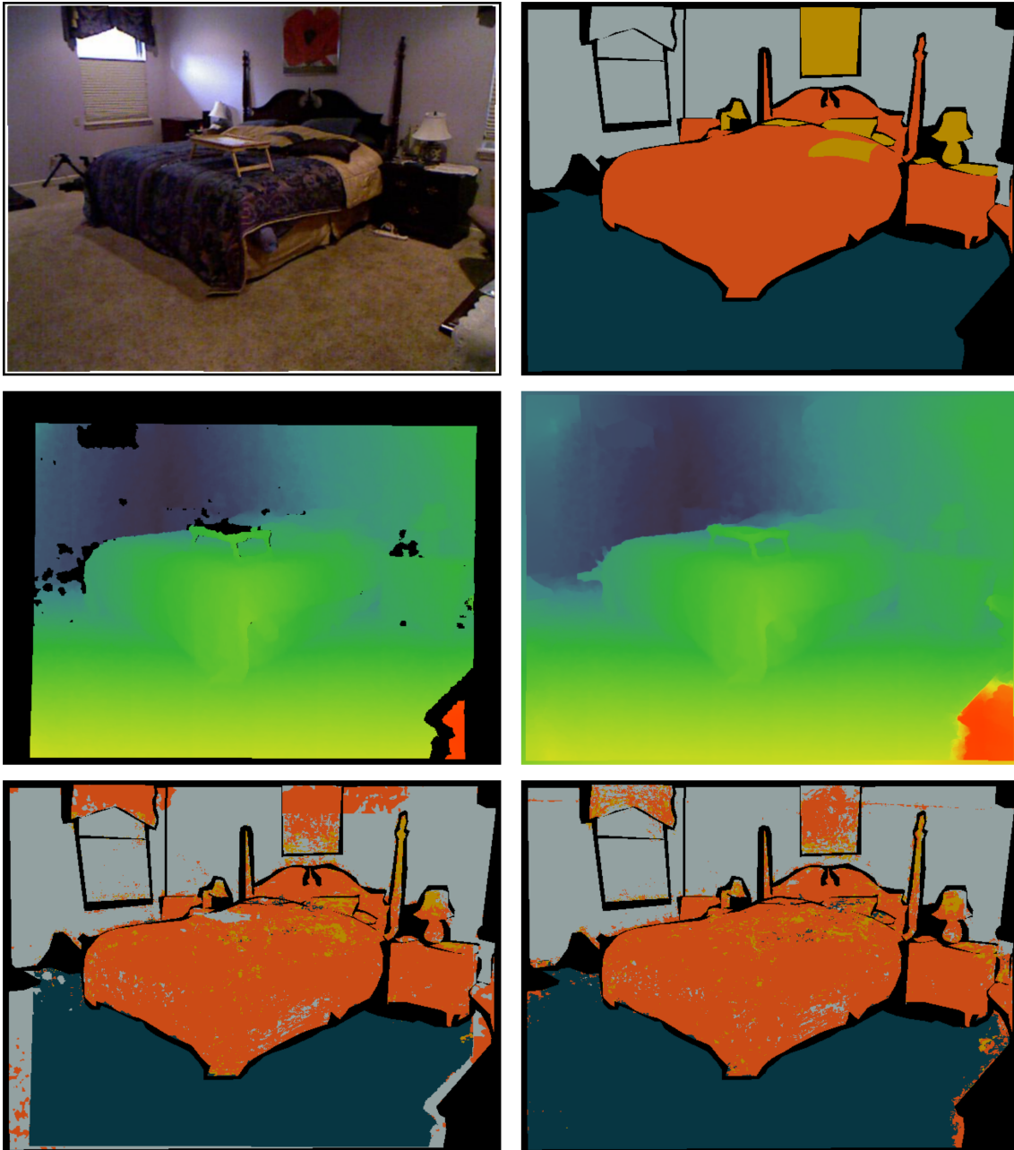
Figure 5.8.: Example of random forest predictions with the raw depth and filled depth version of the NYU Depth v2 dataset. Top left: Color channels. Top right: Ground truth. Middle left: Visualization of the raw depth channel. Black color indicates missing depth. Middle right: Visualization of the filled depth channel. Bottom left: Prediction with raw depth (Pixel accuracy: 87.0%). Bottom right: Prediction with filled depth (Pixel accuracy: 91.4%). Black in the bottom row indicates “void” in the ground truth. Raw depth causes more frequent misclassifications in areas where depth information is missing.
